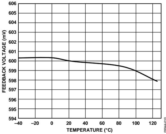
Figure 10. Feedback Voltage vs. Temperature,  $V_{IN} = 3.3\text{ V}$
