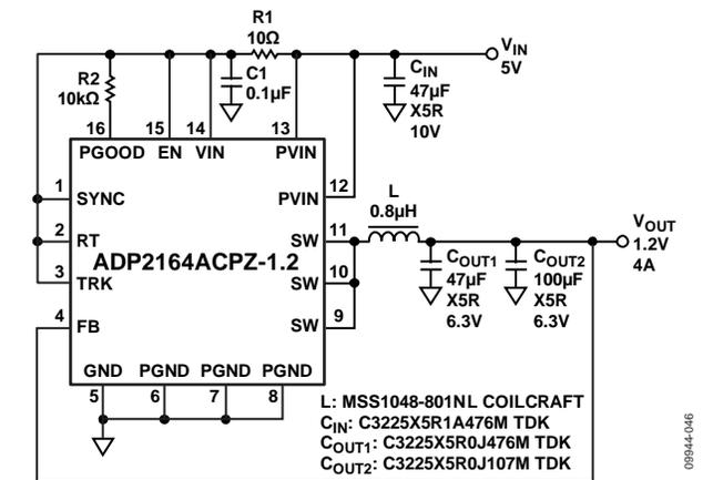
Figure 44. Fixed 1.2 V, 4 A, 1.2 MHz Step-Down Regulator
