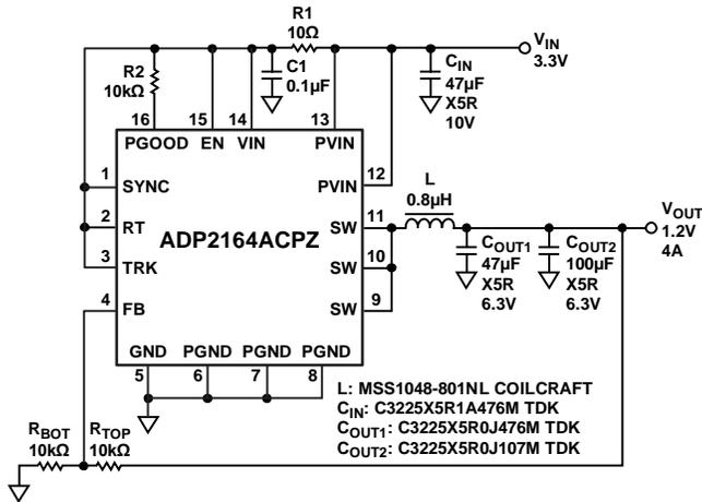
Figure 42. 1.2 V, 4 A, 1.2 MHz Step-Down Regulator
