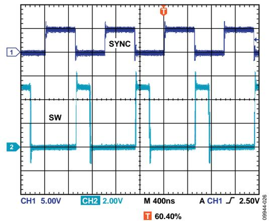
Figure 26. ADP2164 Synchronized to 1 MHz, 180° out of Phase
