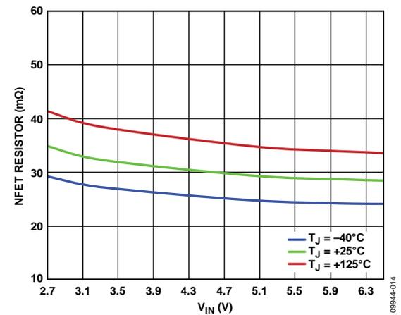
Figure 14. NFET Resistor vs.  $V_{IN}$  (Pin-to-Pin Measurements)
