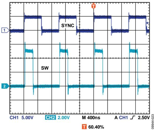
Figure 23. ADP2164 Synchronized to 1 MHz, in Phase
