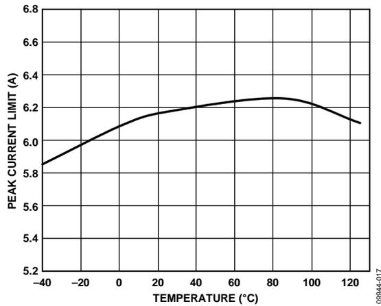
Figure 17. Peak Current Limit vs. Temperature,  $V_{IN} = 3.3$  V
