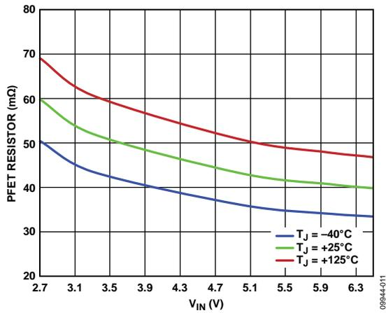
Figure 11. PFET Resistor vs.  $V_{IN}$  (Pin-to-Pin Measurements)
