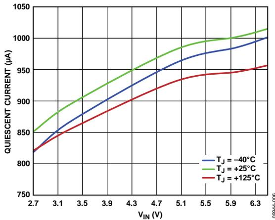
Figure 6. Quiescent Current vs.  $V_{IN}$  (No Switching)
