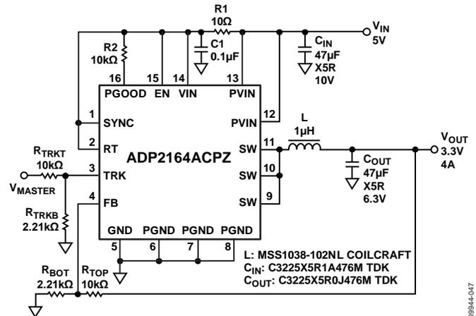
Figure 47. 3.3 V, 4 A, 1.2 MHz Step-Down Regulator, Tracking Mode
