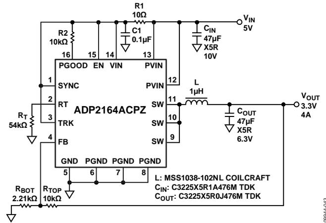
Figure 45. 3.3 V, 4 A, 1 MHz Step-Down Regulator
