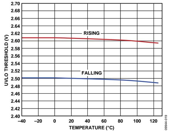
Figure 19. UVLO Threshold vs. Temperature,  $V_{IN} = 3.3$  V
