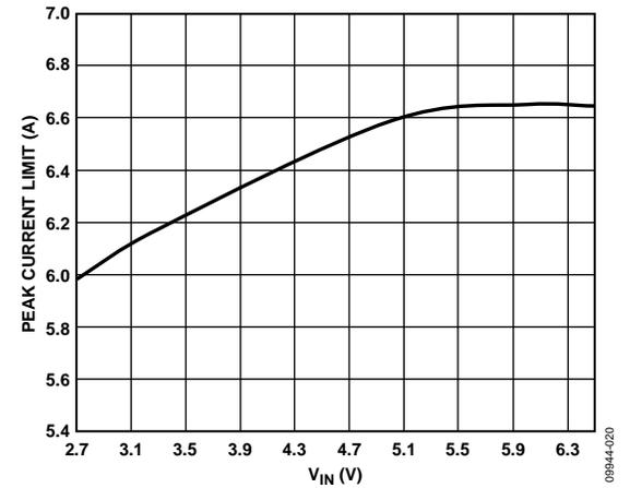
Figure 20. Peak Current Limit vs.  $V_{IN}$ ,  $T_J = 25^\circ\text{C}$
